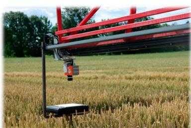
Figure 5. HSI set-up for field analysis.
