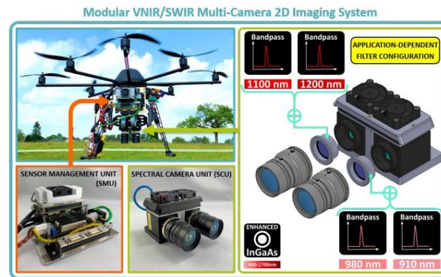
Figure 1: Schematic system overview (See Ref [1])
