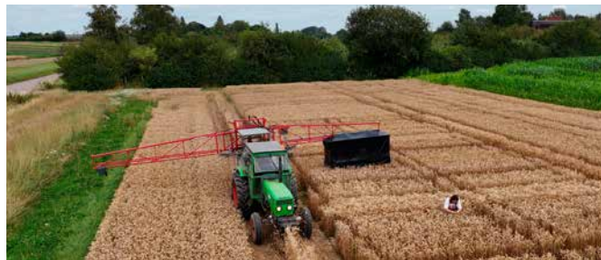
Platform mounted on a tractor for hyperspectral imaging by the CRA-W
