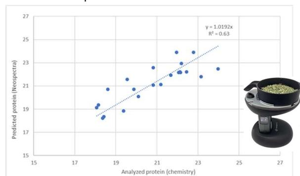
Figure 2 : Protein content prediction (in % of dry matter) with the Neospectra (Si-Ware Systems) on a validation set of 22 samples
