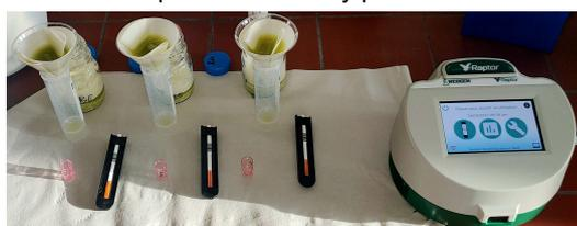
Figure 3 : Reveal® Q+ Max for Ochratoxin A and Raptor Reader
