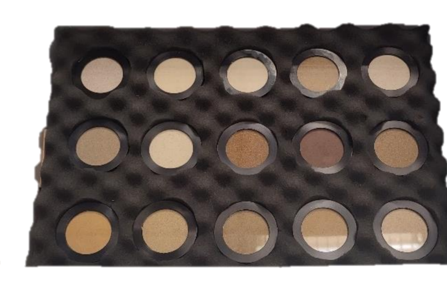
(A) Standardization box sent by CRA-W to laboratories. The box contains 40 samples (30 samples used for standardization and 10 wheat samples used for validation). The samples are presented as sealed cups and contain different feed samples/ingredients. They are characterized by various spectral signatures.
