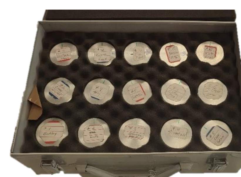
(A) Standardization box sent by CRA-W to laboratories. The box contains 40 samples (30 samples used for standardization and 10 wheat samples used for validation). The samples are presented as sealed cups and contain different feed samples/ingredients. They are characterized by various spectral signatures.
